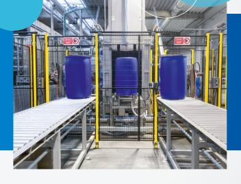
The new system also provides a crucial customer benefit: more reusable plastic drums are available thanks to optimised washing and drying processes. The washing line offers a wide range of programmes and is optimally designed to treat acids, alkalis and oxidising substances as well as finished products such as detergents and lubricants. This range of treatment options means that significantly more empty drums can be processed than previously.
