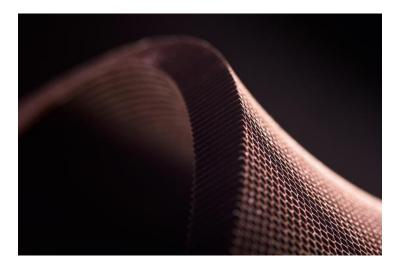
**Caption:** The modern honeycomb material CORMASTER<sup>®</sup> is based on aramid paper and is used wherever low weight and maximum stability are required.
