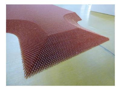
**Caption:** Schütz is exhibiting the CORMASTER<sup>®</sup> honeycomb material at JEC World, a high-tech product that can be shaped into a wide variety of shapes thanks to its excellent processability, making it suitable for a wide range of applications.
