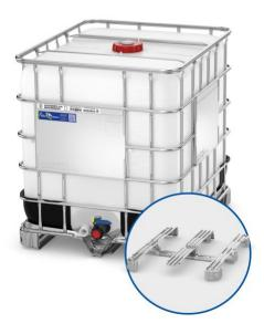
**Caption:** The 3-skid steel pallet with embossed sheet metal skids has an additional central skid compared to standard steel skid pallets. This ensures improved weight distribution thanks to a wider contact surface.
